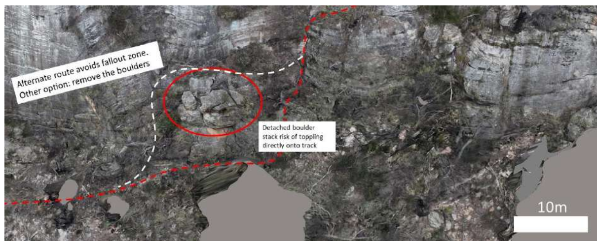
Figure 6-1: Specific large rockfall hazard H1.4 at Section 3 (west)
